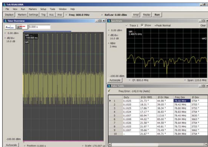
Figure 83. The Spectrum Analysis time window is found to be on just noise.
