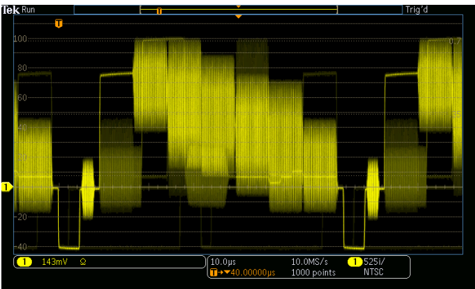
Viewing an NTSC video signal. Notice the intensity-graded view provided by the MDO3000's ability to represent time, amplitude, and distribution over time.
