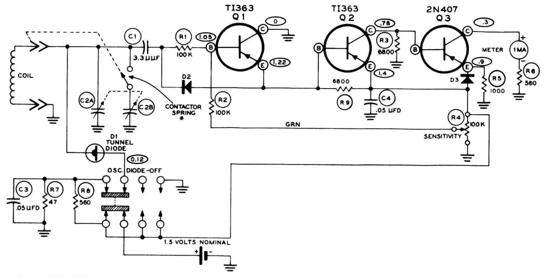
\*C2B SWITCHED INTO THE CIRCUIT BY THE LONGER COIL PLUG PINS.
