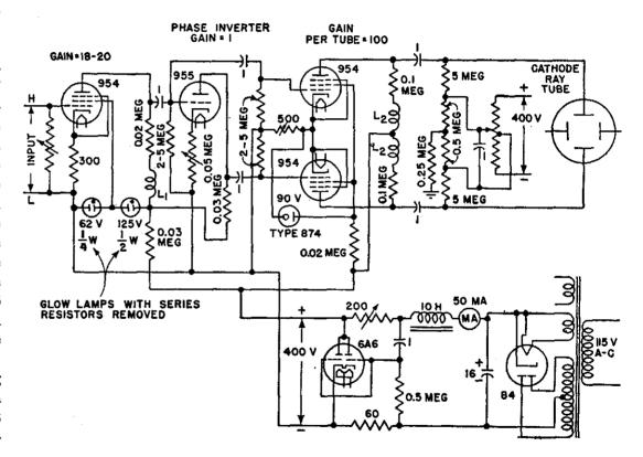
The acorn tubes used combine large mutual conductance with small interelectrode capacitances. They therefore can provide high gain with little phase distortion. The little phase distortion that is produced by the output capaciLarge capacitance values, 1  $\mu$ f, for the coupling capacitors, also contribute to the low phase distortion.
