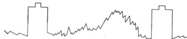
Figure 4 Normal Video and Sync Signal.
