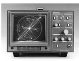
1720 Vectorscope - Vector and Stereo Audio Dual display mode.
