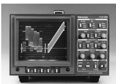
1730 Waveform Monitor - Simultaneous Channel A and B display.
