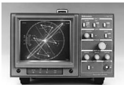
1720 Vectorscope - Vector and Stereo Audio Dual display mode.
