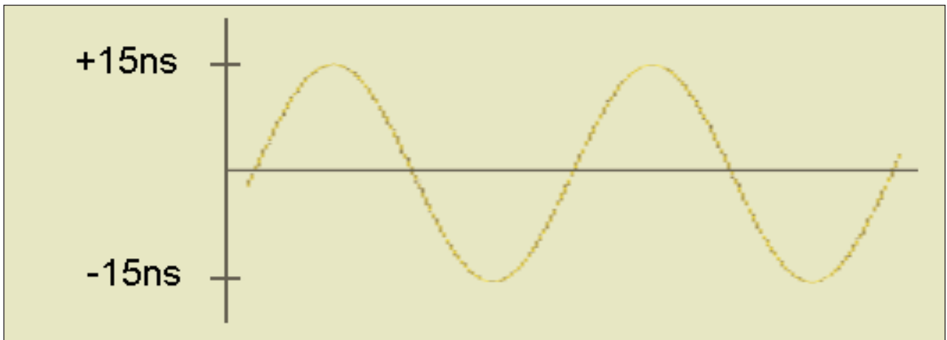
► Figure 3.2c Intended Sinewave Modulation to Apply to a Data Signal
