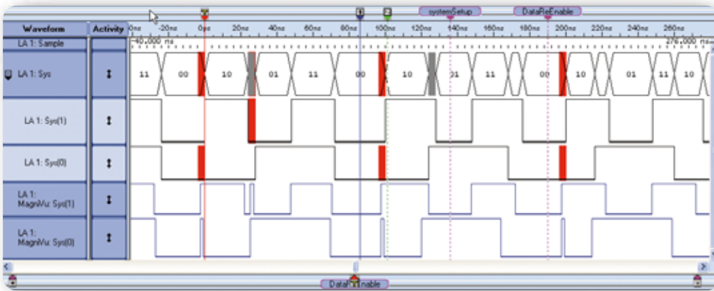
► Figure 21. MagniVu acquisition unveils glitch details by using high-resolution timing waveforms.
