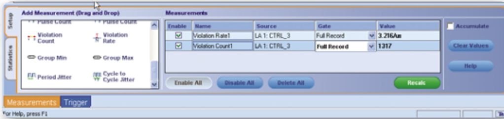
► Figure 17. Automated measurements identify the violation counts and rates.
