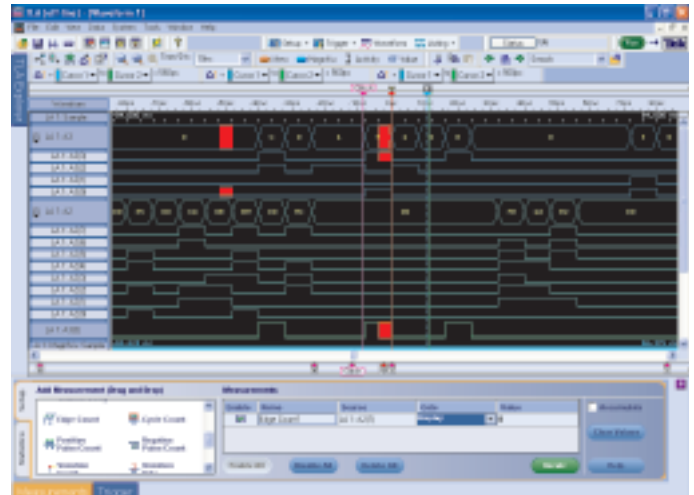
Figure 8. Logic analyzer display showing a timing diagram.
