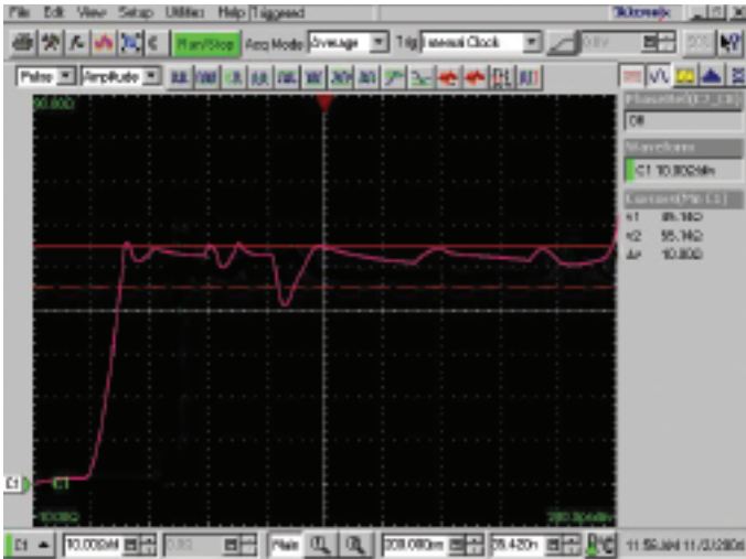
Figure 18. TDR impedance measurement screen.
