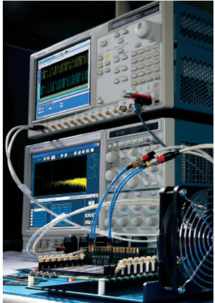
Figure 21. Most measurements require a solution made up of a signal generator paired with an acquisition instrument. Triggering connectivity simplifies capturing the DUT output signal.
