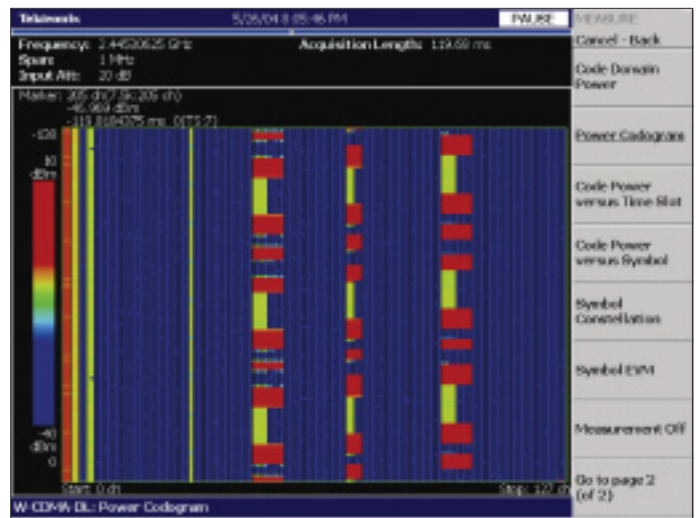
Figure 3-20. Codogram measurement of W-CDMA compressed mode.
