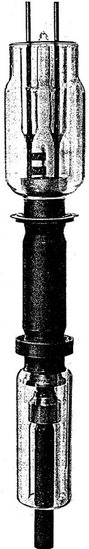
AW-200 HIGH POWER TUBE FOR CYCLOTRON OSCILLATORS.
