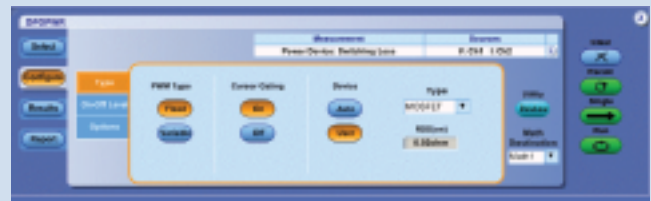
Figure 7. The DPOPOWER input page allows the user to enter data sheet values for R_{DS_{ON}} & V_{CE_{sat}} .
