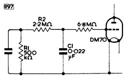
$R_1$  is the load of the demodulator or the A.G.C. diode of the receiver. In addition, in receivers having normal undelayed A.G.C. the decoupling network  $R_2$ ,  $C_1$  already exists and the only additional component is the 6.8  $M\Omega$  resistor. In receivers having delayed A.G.C. it is necessary to control the DM70 from the demodulator circuit. The decoupling network  $R_2$ ,  $C_1$  is then added to the 6.8  $M\Omega$  resistor.
