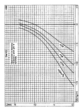
LENGTH OF FLUORESCENT COLUMN PLOTTED AGAINST GRID VOLTAGE AT VARIOUS VALUES OF ANODE VOLTAGE WHEN CONNECTED IN BATTERY-OPERATED RECEIVERS (PIN 5 EARTHED.)
